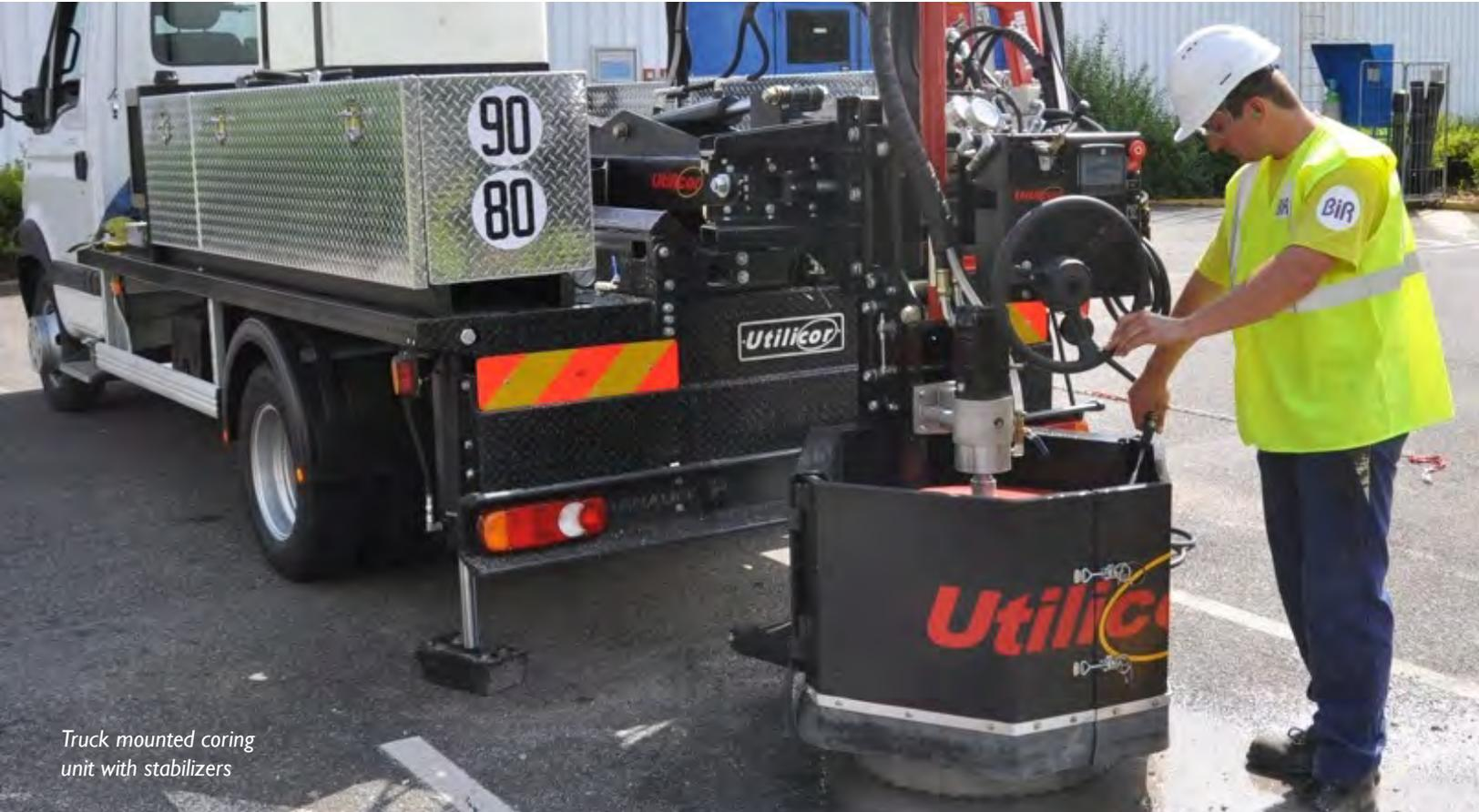
Truck mounted coring unit with stabilizers
