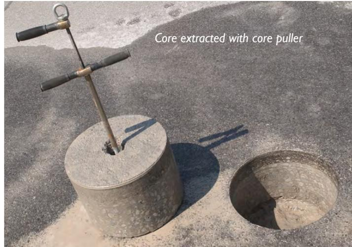
Core extracted with core puller
