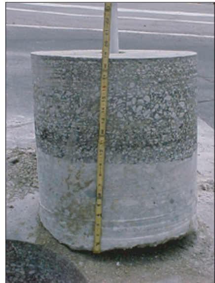
After completing the underground pipe repair, the Nicor crew reinstated the massive 19-inch composite, asphalt and concrete core using Utilibond for a permanent pavement repair
