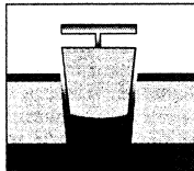
Truck-mounted rotary cutting unit cores a circular hole in the pavement
