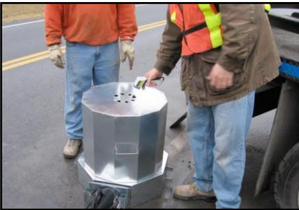
Check the temperature occasionally with a non-contact infrared temperature sensor.
