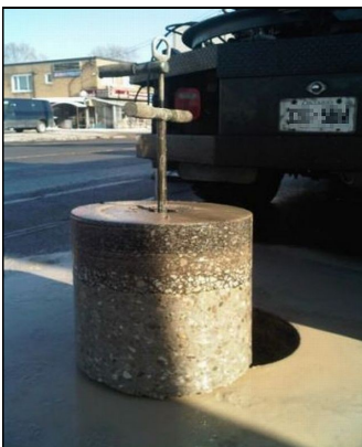
17” deep core pulled from the streets of Toronto
